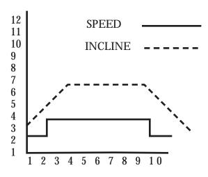
The **Warm Up Program** is designed to gradually increase the treadmill Speed and Elevation in the first segment (warm up) and gradually decrease the treadmill Speed and Elevation in the last segment (cool down). This is also known as a Plateau program.
